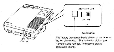
**EXAMPLE:** If the factory preset number is "4", then your code number may be either "42" or "48", depending on the position of the selectable REMOTE code switch.
